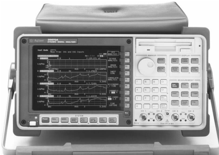
FIGURE C.2 Photograph of the HP 35670A Dynamic Signal Analyzer. (Courtesy of Agilent Technologies Inc., Palo Alto, CA.)
